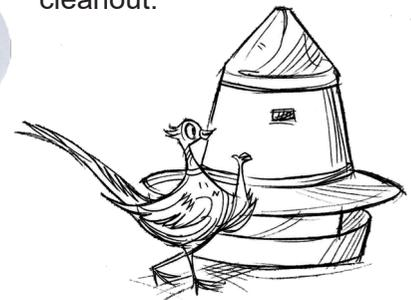
Add capacity with GBF1520 Poly Extension. Add-on shell fits over the rain shield. The top poly shell fits over add-on shell. The shell adds about 17 inches (43.2 cm) of height and about 130 pounds (59.1 kg) of feed capacity depending upon the feed being used. Total capacity with extension is about 305 pounds (138.6 kg).
